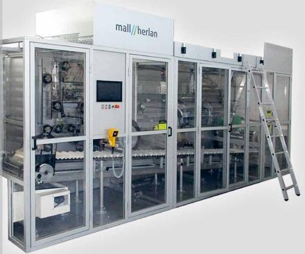
for washing monoblock aerosol cans and bottles made of aluminium or steel after necking
