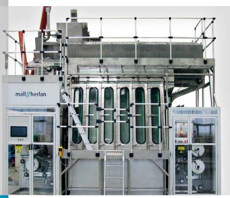
for washing monoblock aerosol cans and bottles made of aluminium or steel
