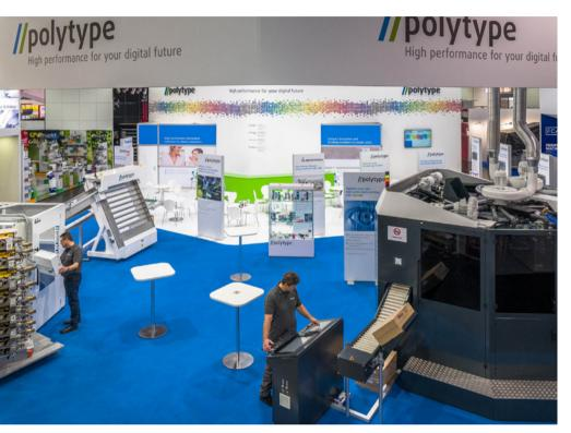
At K 2022, //polytype will present a global innovation and milestone in the production of plastic tubes. A tube becomes a tube when a tube shoulder is applied to a sleeve using compression molding before being capped. The new //polytype HC130 combines these two processes in a single machine. At the K 2022, visitors will have the opportunity to see the revolutionary ORBITdrive concept in action live on the HC130.
