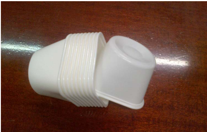
Square-round portion cups, lip rolled OMV has successfully tested its proprietary lip rolling system on various square cups and trays
