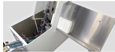
The //polytype BDM 301 is equipped with cup feeding with worm infeed. Corona pre-treatment is split between two separate stations – one for the side wall and one for the bottom. Transfer, cup positioning before and after printing, and universal cup take-off are included as standard.
