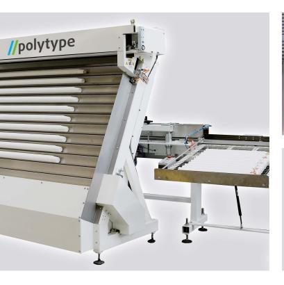
The wide in-feed elevator (2.1 m) with high storage capacity and electronic pusher ensures controlled pressure of cups to feed scrolls. A protective enclosure enables excellent access to the print and transfer areas. The process ends with a discharge table with a precise laser counting device.
