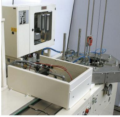
The //polytype DDM 160 ensures quick and easy format changes thanks to its excellent accessibility. One-man operation is supported by an infeed robot comprising conveyor belt, feed module and multi-stack elevator. Tooling changes on the feeding scrolls are also made easier thanks to the automatic lift-up scroll feeder.
