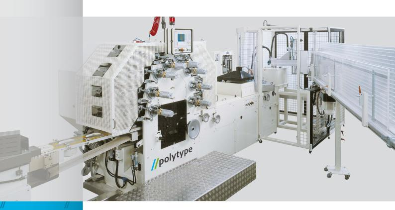
The //polytype DDM 160 is equipped with antighosting inking units with an ink agitator and leakfree ink fountains that can be removed quickly. A separate drive makes for quick and easy automatic roller cleaning and pre-inking. Ductor roll cooling is available as standard, oscillator roll cooling as an option.
