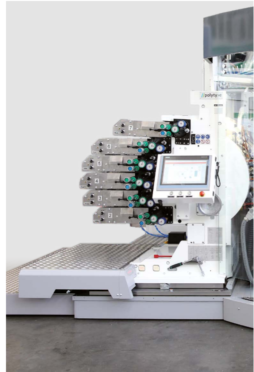
The dry offset printing unit T80 for small diameters
