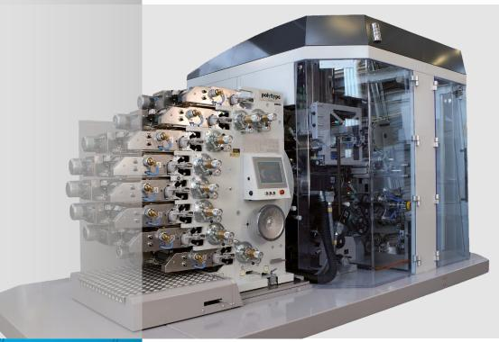
The high-performance offset printing, lacquering and finishing machine for plastic tubes
