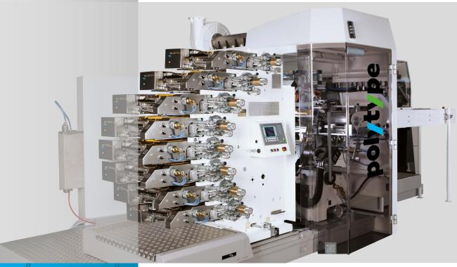
The compact offset printing, lacquering and finishing machine for plastic tubes
