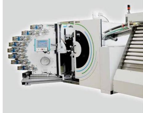
The //polytype BDM 681/682 is very user-friendly and designed for one-man operation. All main components are easily accessible and every inking unit can be swung out individually. Functions such as automatic washing and pre-inking of inking units are available to cut changeover times. All register settings can be made on the fly.
