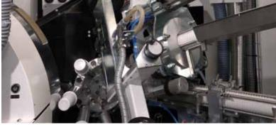
The wide in-feed elevator (2.1 m) with high storage capacity and electronic pusher ensures controlled pressure of cups to feed scrolls. A protective enclosure enables excellent access to the print and transfer areas. The process ends with a discharge table with a precise laser counting device.
