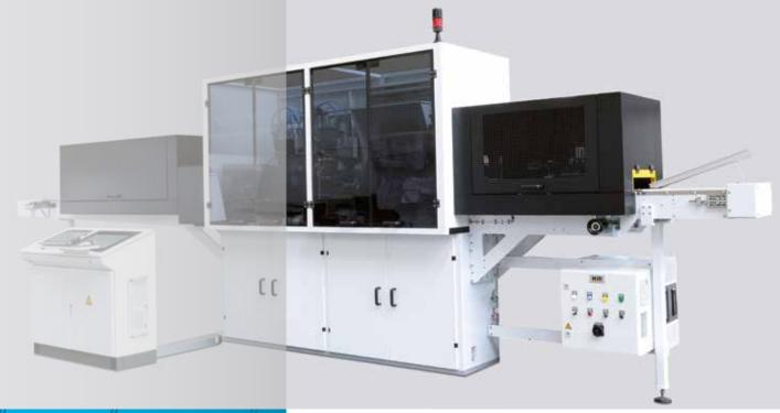
The universal digital printing machine for flat surfaces
