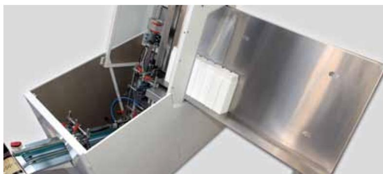
//polytype BDM 301 is equipped with cup feeding with worm infeed. Corona pre-treatment is split between two separate stations - one for the side wall and one for the bottom. Transfer, cup positioning before and after printing and universal cup take-off are included as standard.
