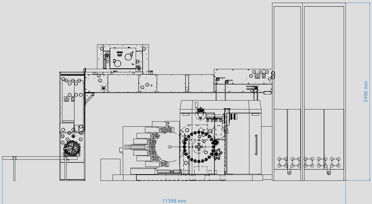
The //polytype RDA 24-165 is a 2-in-1 high-performance offset printing and lacquering machine for inline and offline production. It enables complete finishing for tubes on an extremely small footprint.
