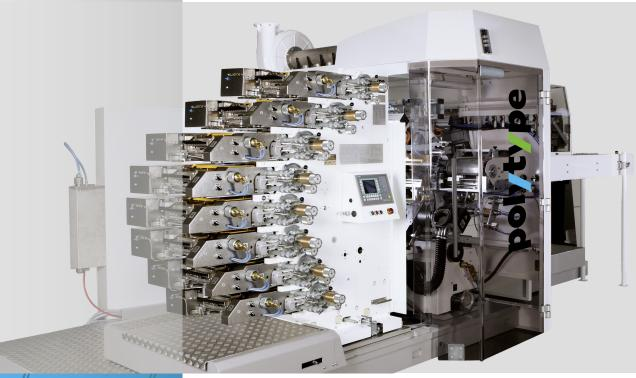
The compact offset printing, lacquering and finishing machine for plastic tubes
