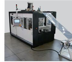
F25/5 The universal thermoformer Forming sizes: 850 x 250 mm single rows stacking device
