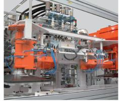
E76 High production thermofomer for OMV international patent «shuttle mould» forming technology Forming sizes: 760 x 540 mm
