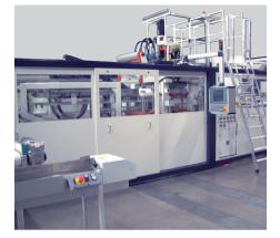
F37 and F37X The medium/large universal thermoformer Forming sizes:  $F37 = 780 \times 420 \text{ mm}$  $F37X = 800 \times 550 \text{ mm}$
