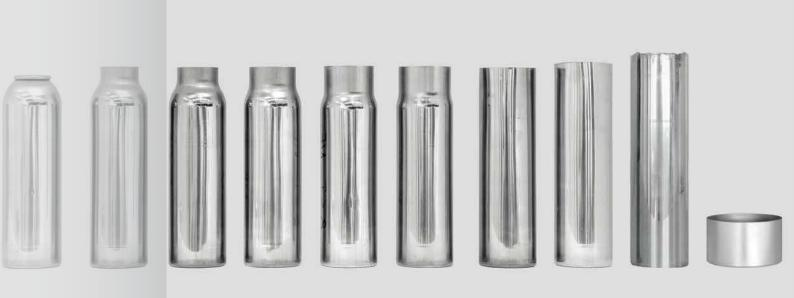
For monoblock aerosol steel cans, //xtracan is setting highly modern standards with its new DWI Line. In the frontend a steel cup is punched out of a steel coil and the cup is then ironed into a cylinder in the bodymaker. The cylinder is directly transfered into the integrated decoration unit with inside coating and up to 9 colour printing machine. Even digital printing is possible. With a modular necking system the can is necked to its individual style.
